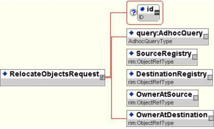
Figure 84: RelocateObjectsRequest XML Schema
