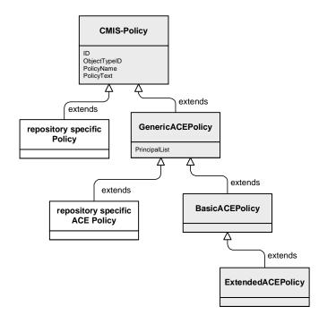
ACEs for Level-1-ACLs should have a type inheriting from GenericACEPolicy assigned. ACEs for Level-2-ACLs should have a type inheriting from BasicACEPolicy (to denote a basic permission, or ExtendedACEPolicy to denote an extended permission).
