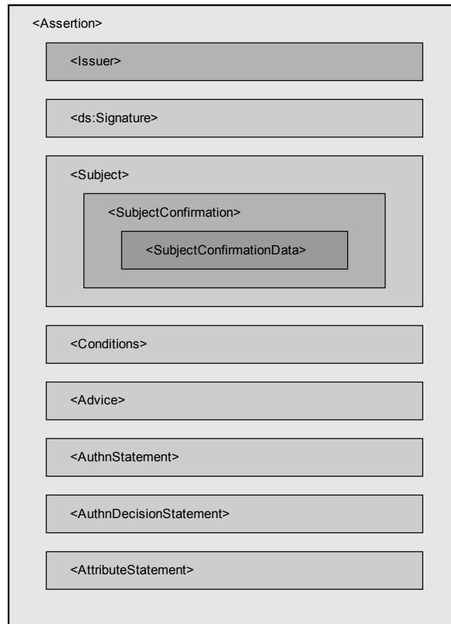
Figure 3: Structure of a SAML 2.0 Assertion
