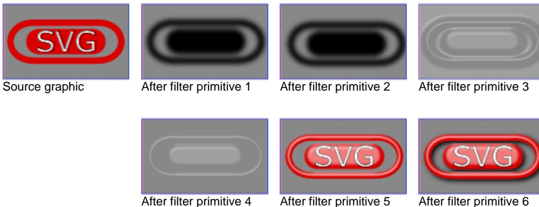
1. Filter primitive **'feGaussianBlur'** takes input **SourceAlpha**, which is the alpha channel of the source graphic. The result is stored in a temporary buffer named "blur". Note that "blur" is used as input to both filter primitives 2 and 3.
