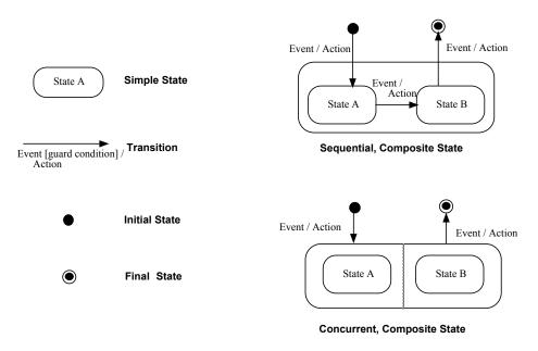
Figure 12 - UML State Diagram Notation
