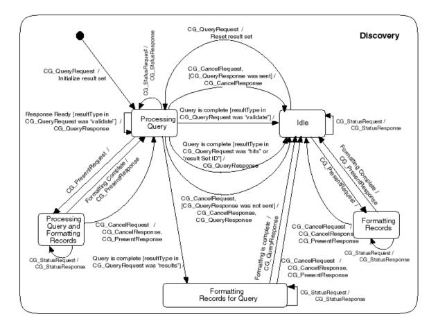
Figure 15 - Discovery State Diagram (Complete)
