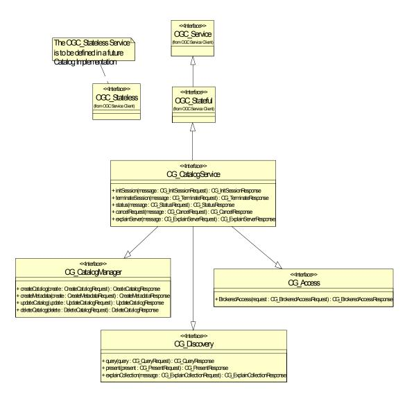
Figure 7 - Main Static Class Diagram of the General Interface Model
