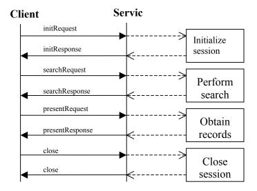
Figure 21 - Z39.50 Profile Sequence Diagram
