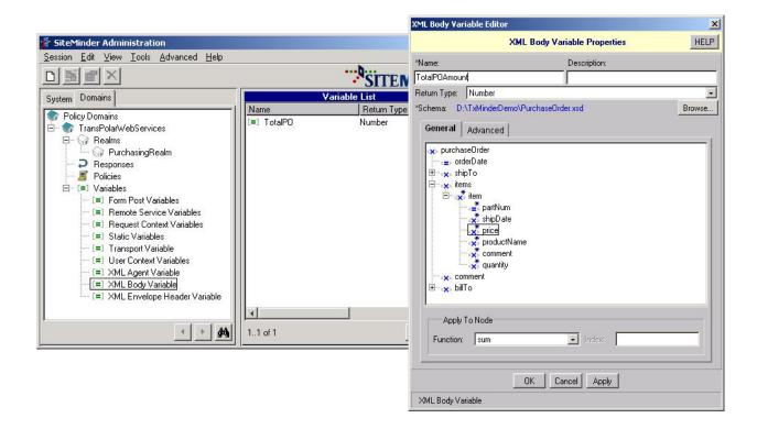
In this example we're creating an XML Body Variable. The Web service provider has defined the format of the business payload in an XML schema. In this case, the business payload is a purchase order (PO). We pick the desired field from the PO XML schema ("price", in our example) that will be evaluated at runtime.
