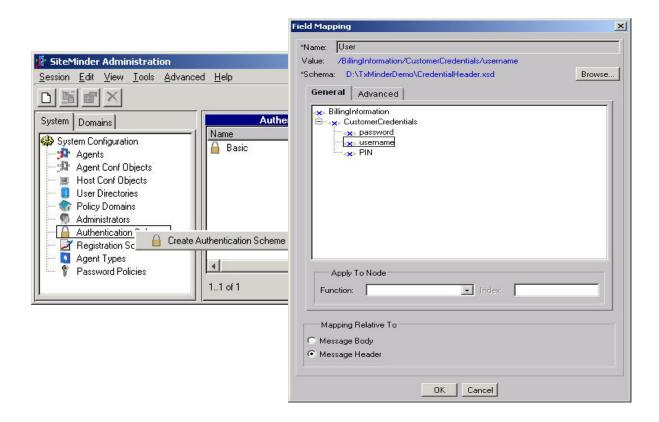
The Web service provider defines the format of a SOAP header that contains the credentials. In this example, we use a username / password authentication scheme, but we could use other variations including a PIN as shown in snapshot above.
