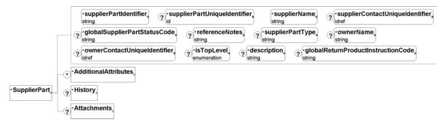
Each supplier part is represented by a SupplierPart element. A supplier part element is used to associate suppliers and parts through the use of an approved supplier list. For example, this element could represent a power supply purchased from a list of approved distributors or a spool of resistors purchased from an approved supplier.
