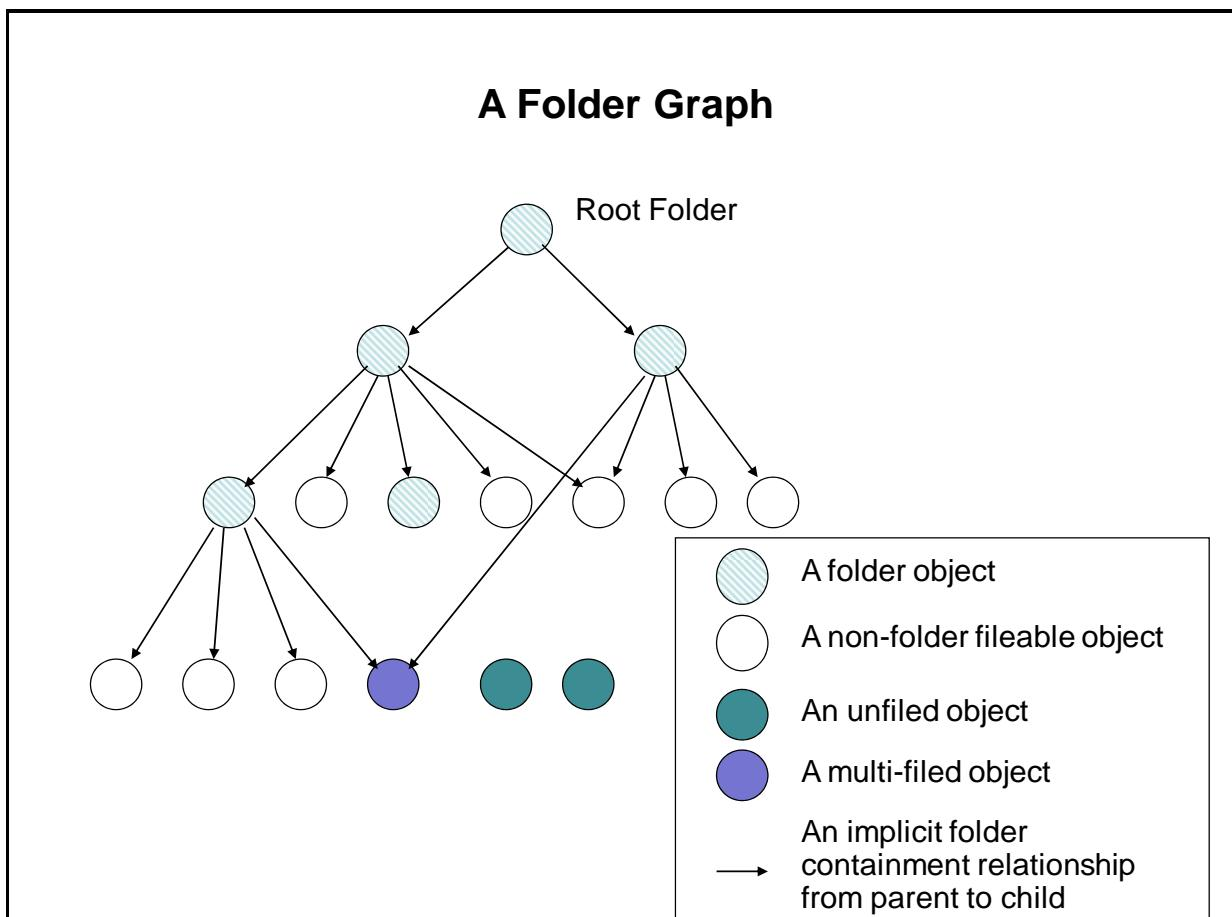
Folder objects are handled using [the basic CRUD services for objects](#), and the folder graph is traversed using the [Navigation Services](#).
