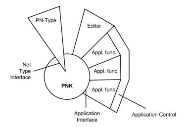
Fig. 4. Conceptual Model of the Petri Net Kernel.
